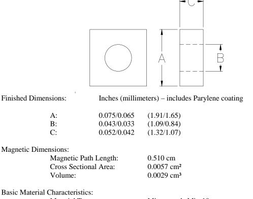
Dasie Material Characteristics:Micrometals Mix-10Material Type:Micrometals Mix-10Initial Permeability:6 (Reference)Temperature Stability:+150 ppm/C typicalFinish:0.001" Parylene C, Clear
