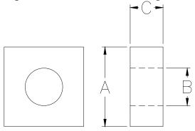
Finished Dimensions: Inches (millimeters) – includes Parylene coating
